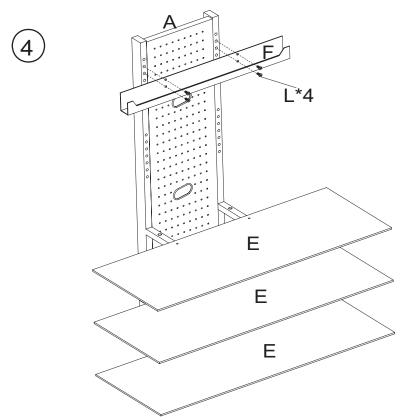
4-Attach holder (F) to panel (A) with screws (L). Place glass (E) on the pads.
